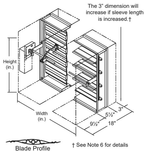
**Smoke Damper ▲ Leakage Class I ▲ Airfoil Blades ▲ 250°F or 350°F Rated ▲ Galvanized Steel**
